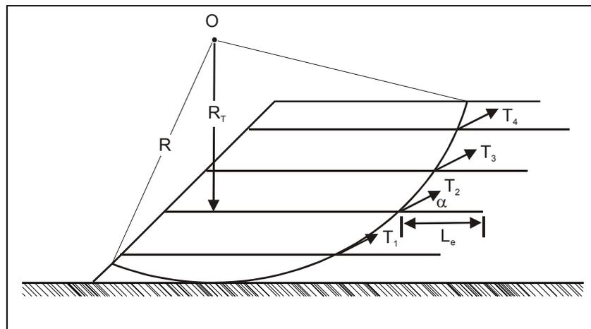
Example circular slip analysis of reinforced soil slope over stable foundation
