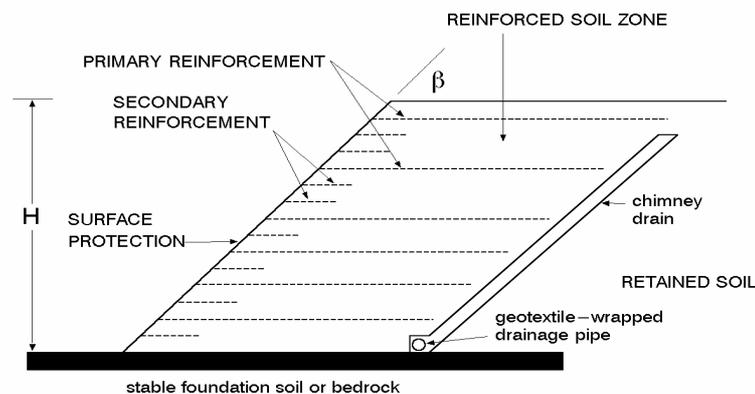
Geosynthetic reinforced soil slope over stable foundation
