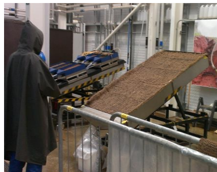
Laboratory testing of geosynthetics using simulated rainfall
