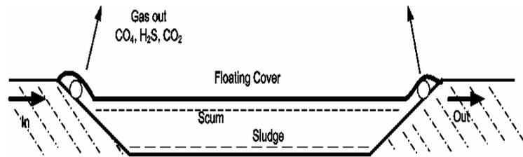
Generally these lagoons will take wastewater with BOD of 400 to 5000 kg/cum and the output effluent will have the BOD reduced by 90 to 95%. Detention time is normally 4 –7 days. The anaerobic process is largely self propelled and the only mechanical input is that required to feed wastewater to the lagoon and force its exit at an overflow outlet. There may
