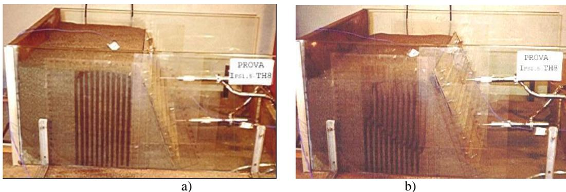
Fig. 1 Shaking table test on a geogrid-reinforced wall model: a) before the shaking; b) after the shaking
