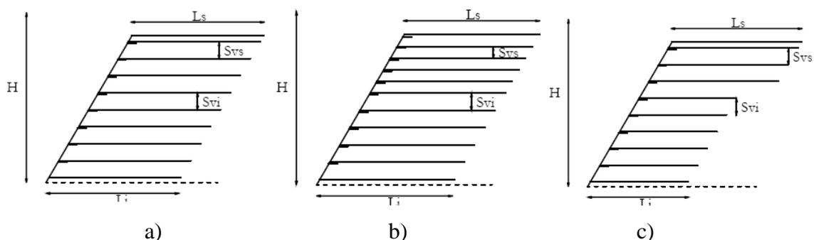
Fig. 2: a) uniform length and uniform spaced reinforcements; b) uniform length reinforcements with reduced spacing at the top; c) uniform spaced reinforcements with increased length at the top.
