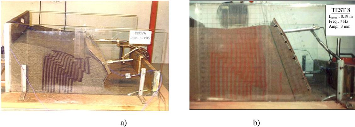
Fig. 3. Response of different reinforced type wall to the same seismic excitation: a) failure of a wall with uniform length and uniform spaced reinforcements; b) acceptable permanent displacement of a wall with uniform length and reduced spacing of reinforcements in the upper part of the wall.
